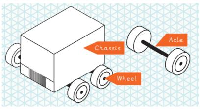
The wheels need to be attached to an axle. The axle needs to fit inside the axle holder but must not be attached to the axle holder or the wheels will not be able to turn properly.
